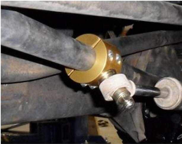
14. Position the clamp so the stud measures 11.5" from the center of the stud to the center of the factory stabilizer mounting hole.
