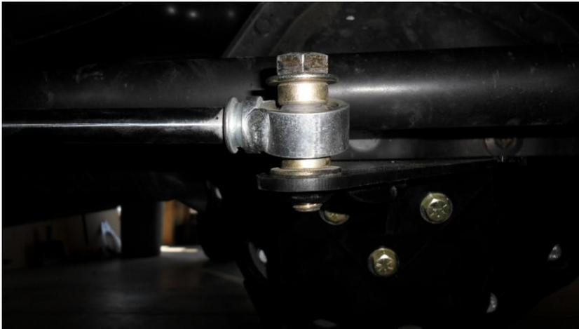
17. When installing the stabilizer onto the Clamp's Stud, install  $\frac{1}{2}$ " washer, then a spacer, then stabilizer, then another spacer, then the  $\frac{3}{8}$ " washer, and finally the  $\frac{3}{8}$ " Nyloc nut.
