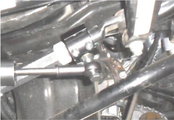
5. **A. Stock Height or Carli Torsion Sway Bar:** Remove the two bolts that hold the sway bar to the frame on the PASSENGER side.
