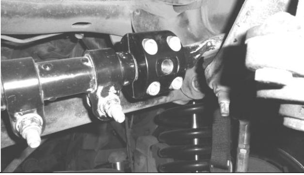
2. Tighten the 4 Allen head screws in a cross pattern with 5/16" Allen Key (8mm also works). Torque bolts to 13ft.lbs.
