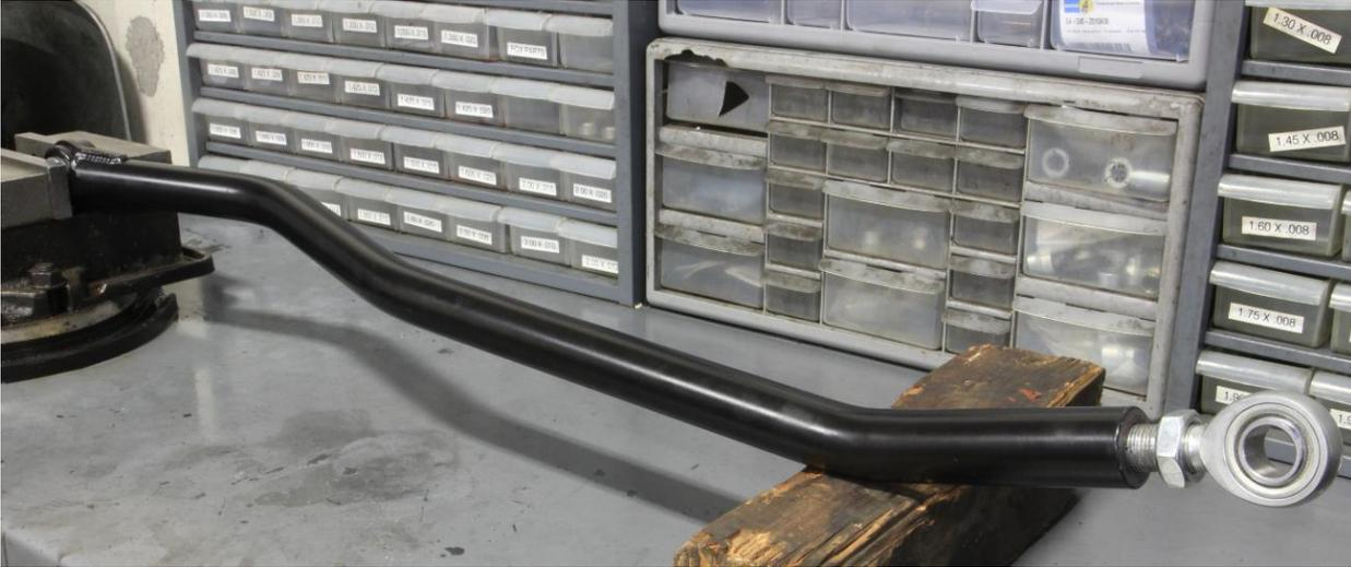
7. For a 2"-3" of front lift, set the Carli adjustable track bar to 39-1/8" from the center of the heim to the center of the uniball.
