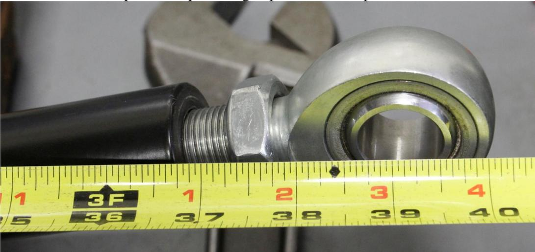
8. **APPLY RED-LOCTITE TO THE THREADS** where the jam nut will assemble to the end of the track bar.
