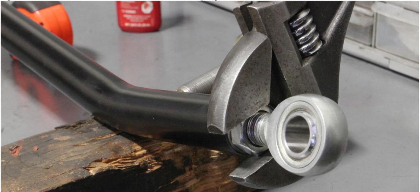
10. Confirm ends remained parallel during torquing.
