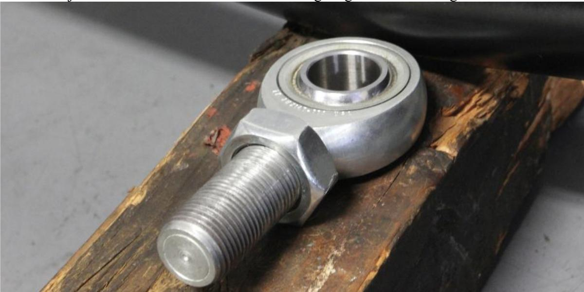
4. Apply a light coat of anti-seize to the last few threads on the rod-end and thread it half-way into the end of the bar.
