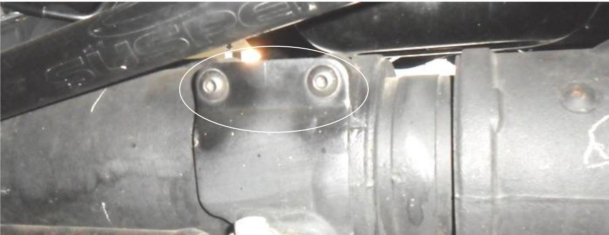
3. Use the provided 1/2" button head bolt to replace the factory axle side steering stabilizer bolt. Ensure the nut faces the ground and torque to 35 ft.lbs.
