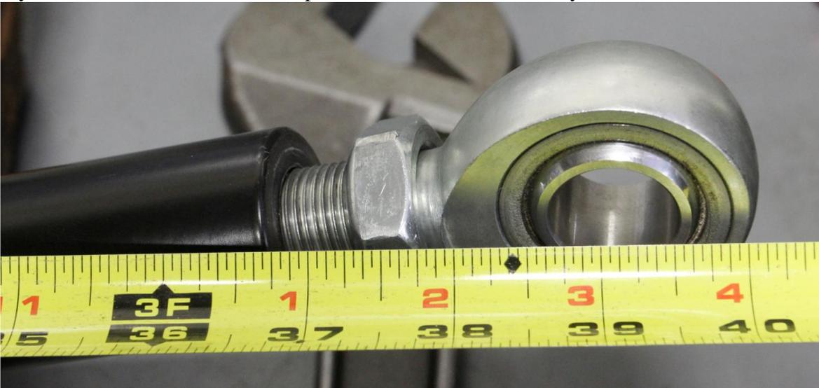
10. **APPLY RED-LOCTITE TO THE THREADS** where the jam nut will assemble to the end of the track bar.
