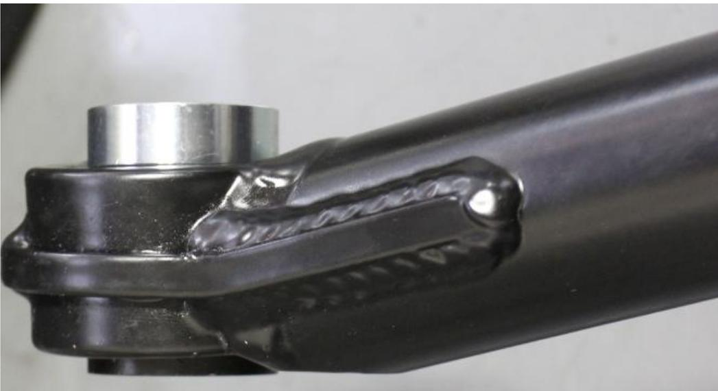
8. Secure the frame end of the track bar (with mis-alignment spacers installed) in a bench vice and use a block of wood to elevate the heim joint (axle) end. (old style Johnny-Joint shown in the picture for reference only).
