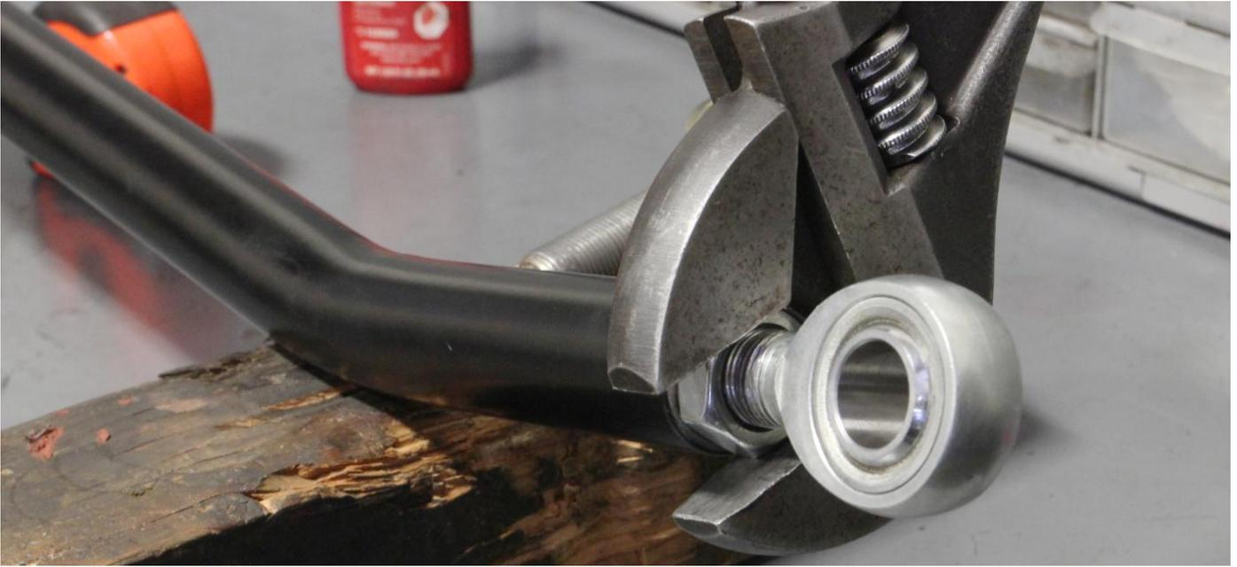
12. Confirm ends remained parallel during torquing.
