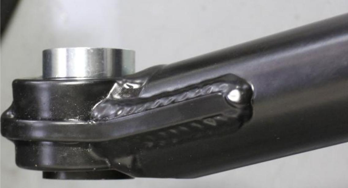
18. Slide the Uniball assembly into the frame side bracket and install factory bolt and nut to secure the uniball.
