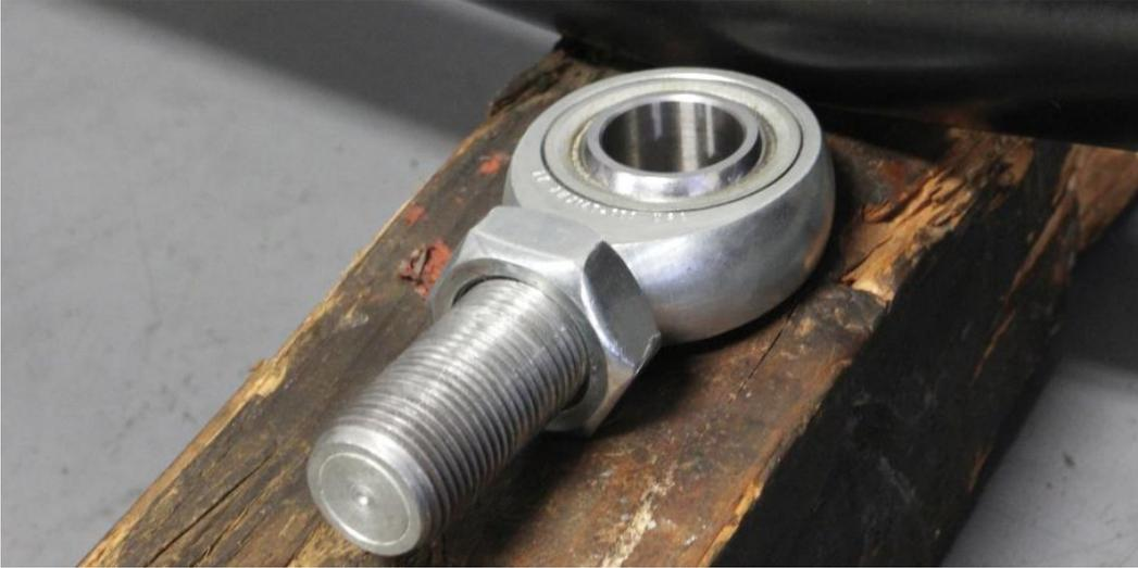
6. Apply a light coat of anti-seize to the last few threads on the rod-end and thread it half-way into the end of the bar.
