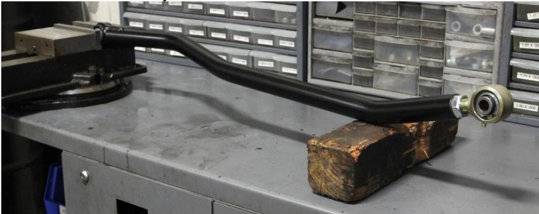
3. Using a torch, heat the threaded end of the bar to melt the loctite applied in the initial installation.
