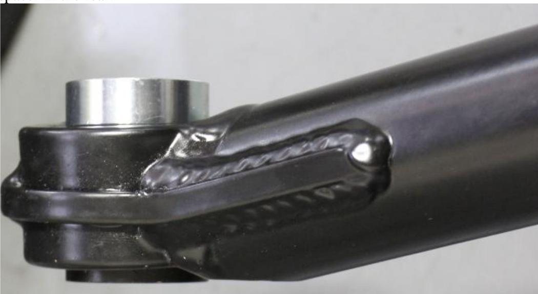
**14.** With the bar now assembled, slide the assembled heim joint with misalignment spacers into the axle pocket and assemble with the factory hardware for torquing later.
